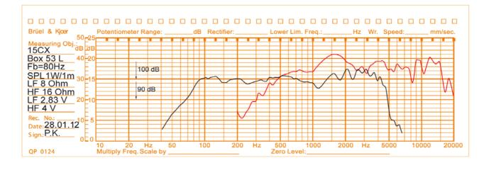
388 mm (15 in) LF 8 Ohm /HF 16 Ohm 6.20 Ohm 50 - 16000 Hz 80 deg
