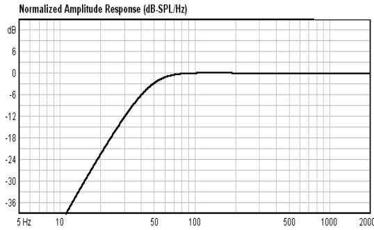
PREDICTED LOW FREQUENCY RESPONSE • Bass-reflex cabinet, Vb=45.00 l, fb=38.0 Hz
