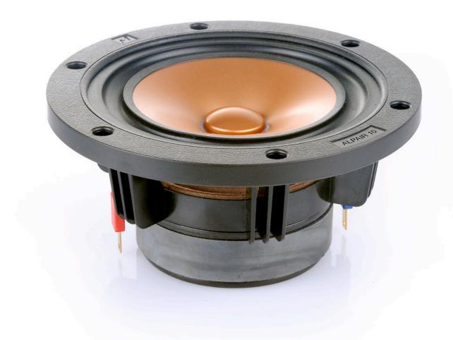
This Alpair 10 is the latest model in a development line designed to extend the performance of mid-sized Markaudio full-range emitters. Measured performance is extended. Vas increases from 21 to 28 litres. Fo is now 36Hz, 4Hz lower than the old model. Total Q increases to 0.33 making this new Alpair 10 usable in larger audio applications.
