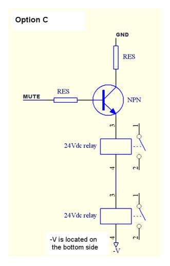
Option C shows how to implement two relays which offers the possibility of more sets of contacts. Note that the circuit now is supplied from the power amplifier supply to ensure enough voltage for the relays.
