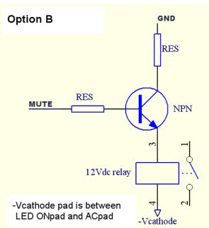
Option B shows the circuit with a relay output. The relay can have more than the one set of contacts shown on the schematic which make it possible to control either signal input or output of the amplifiers.
